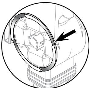
Make sure the **handle** is tight to the body, positioned above side notch.
