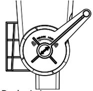
Push pin in. Rotate to the locked position.
