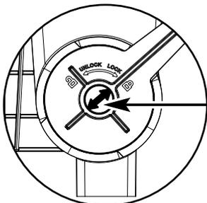
Make sure the **handle** is installed correctly with the pivot pin locked in place.
