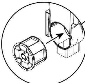
Make sure the **friction pad and cylinder** are properly installed.
