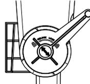
Align arrow on the pin with the unlock position.
