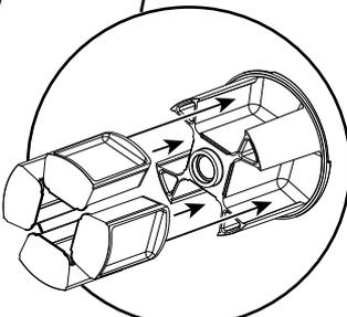
Make sure the **portion trays** are installed correctly. The curved tab on tray end should rest outside cylinder.
