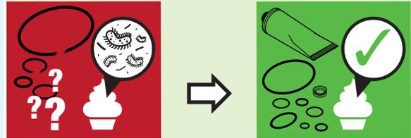
Kit of scrapers to ensure the best cooling efficiency and quality of the product. Worn scrapers increase product dispensing time and recovery time. Replacement is required every 6 months.
